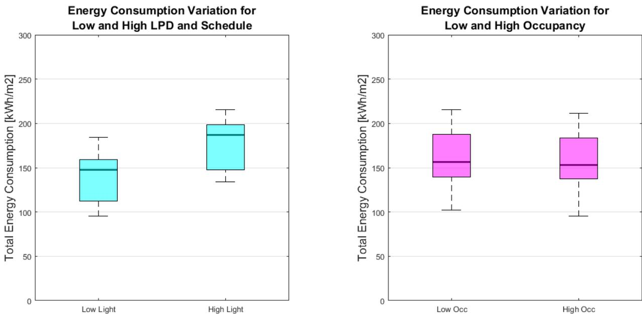
Fig. 7: Variations in total energy consumption due to high/low lighting power density and use behavior (left) and due to high/low occupancy (right)
