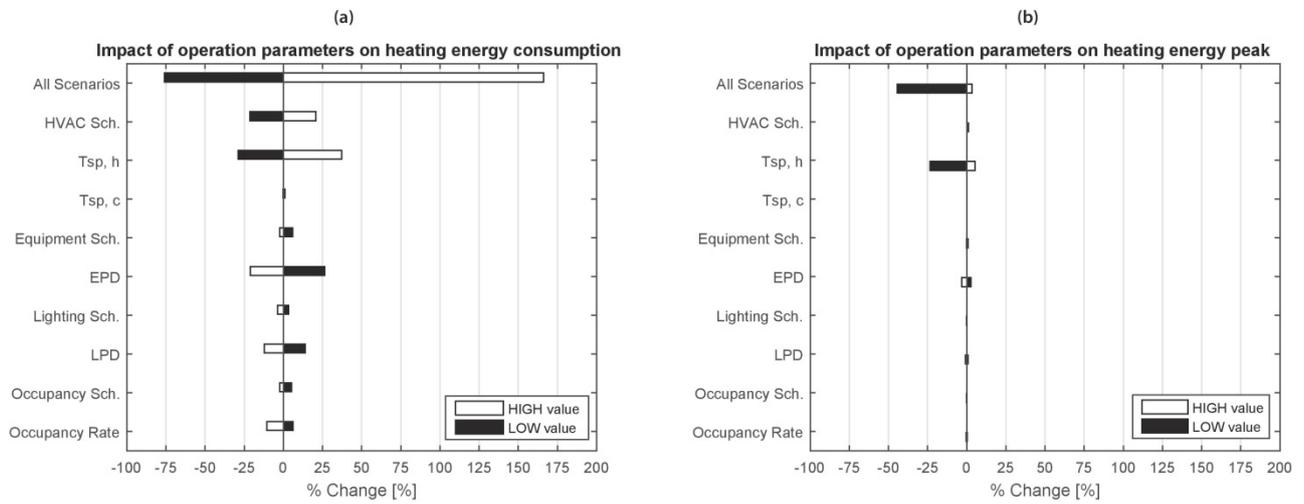
Fig. 6: Variations in heating energy consumption (a) and heating energy peak (b) due to operation scenarios
