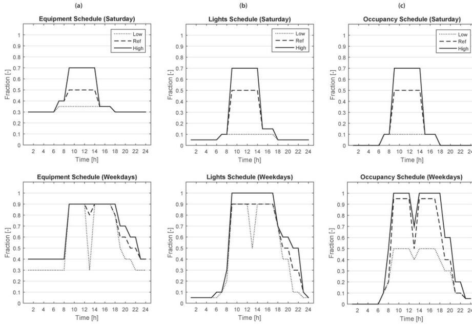
Fig. 5: Low, reference and high schedules for equipment use (a), lights use (b) and occupancy (c)
