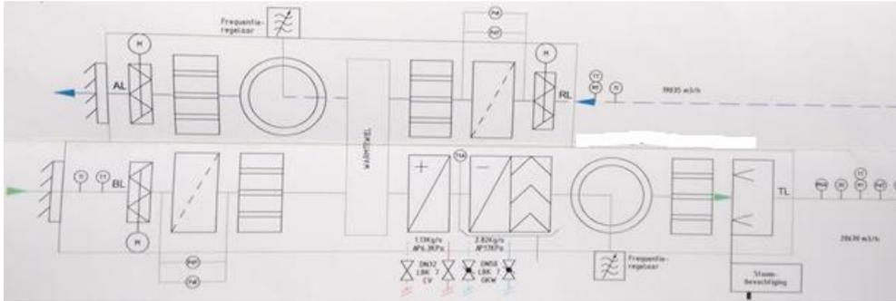
Figure 1. Schematic of the Air-Handling unit from the TRECO-office case-study building
