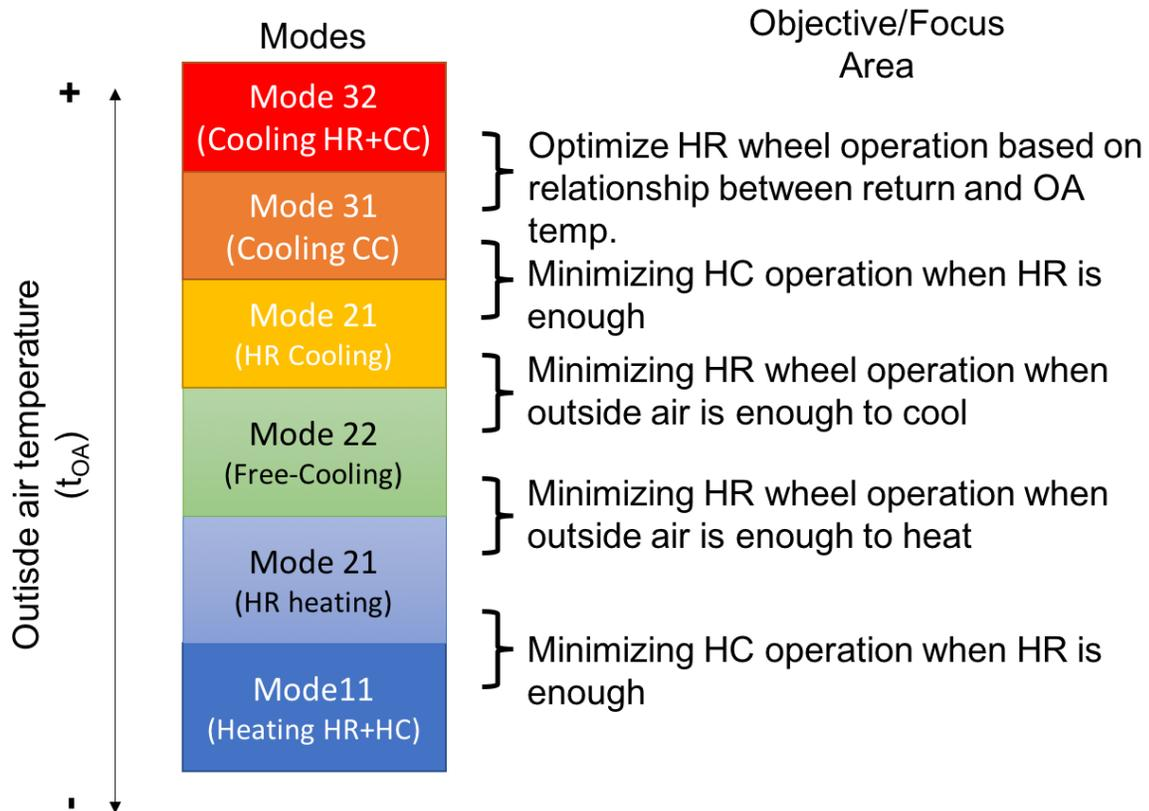
Figure 3. AHU Operation modes and objectives
