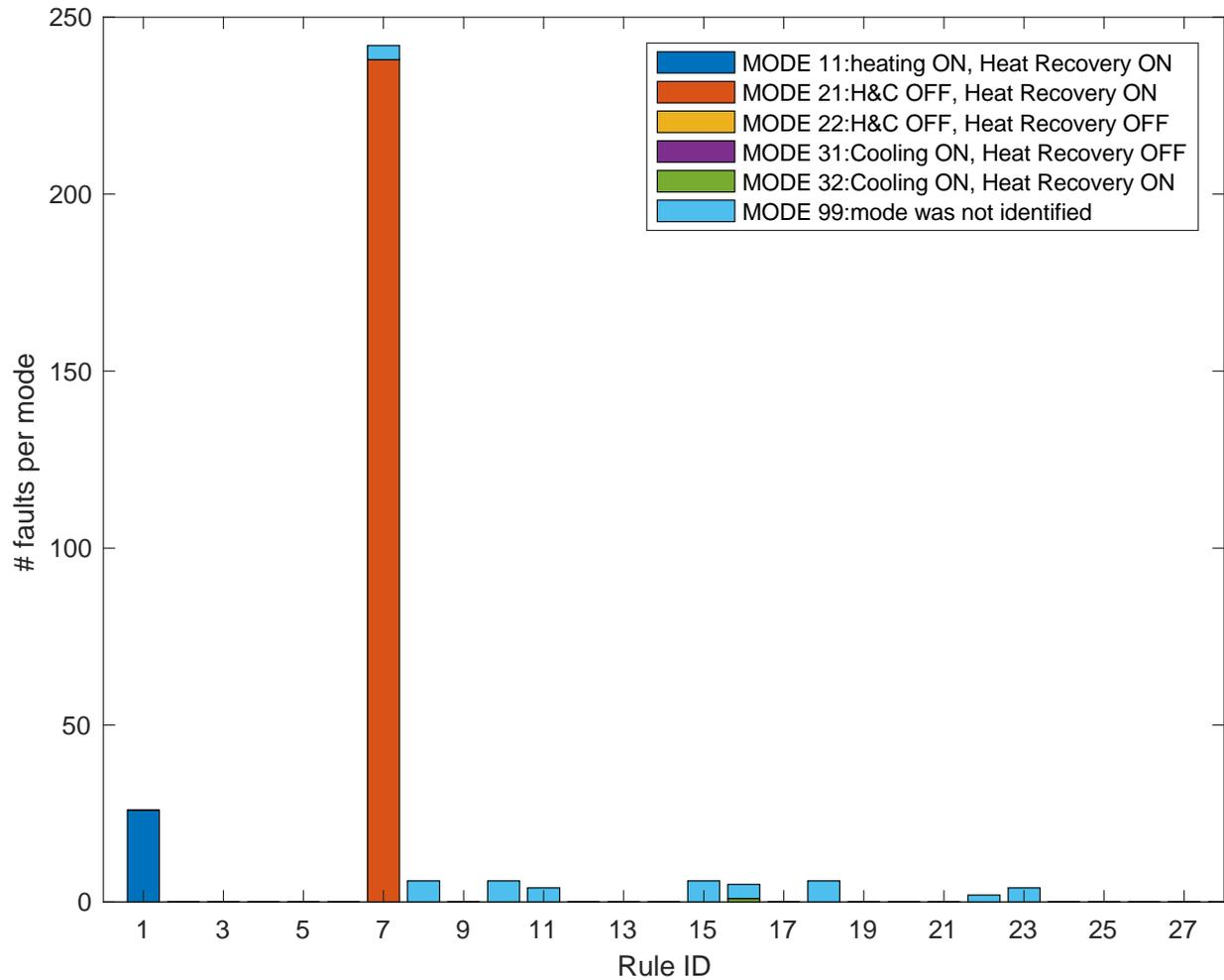
Figure 5. Faults triggered based on rule ID and AHU operation mode for December
