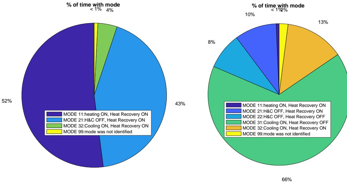
Figure 4. Time spent in AHU operation modes for December (left) and August (right)
