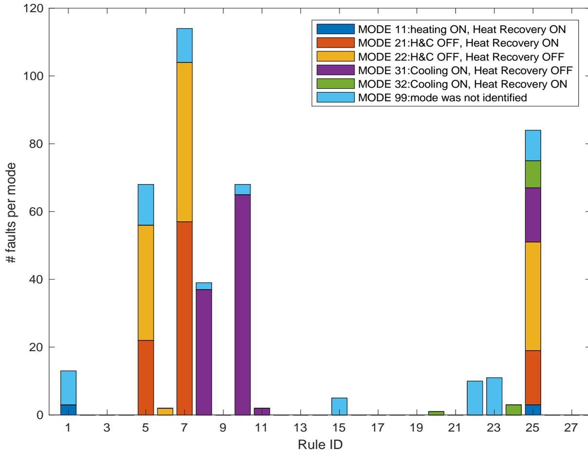
Figure 6. Faults triggered based on rule ID and AHU operation mode for August
