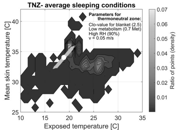
Figure 7, Contourplot of measurements including the calculated TNZ for this test-subject with parameters that should represent the micro climate in bed
