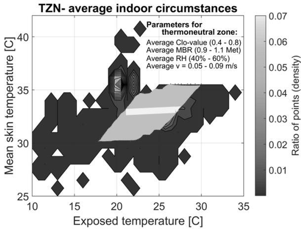
Figure 8, Contourplot of measurements including a range of calculated TNZ's for this test-subject with parameters that should represent the indoor environment
