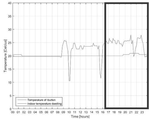
Figure 9 Temperature logged by the iButton on the outer side of the clothes versus the temperature logged by the dwelling. The orange window indicate the moment when the test-subject was present
